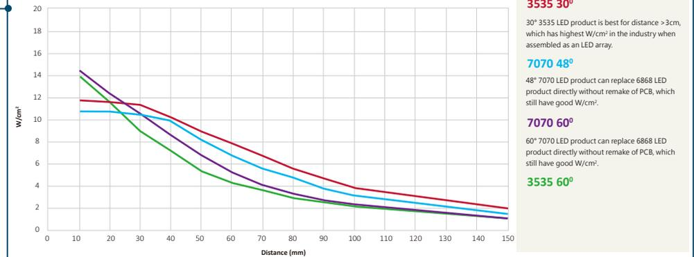
Remark : 1. Industry standard EIT UV Illuminometer    2. Value of UVA, UVB value is added    3. LED array refer to ProLight's standard module    4. Test time < 3sec
